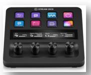
The devices feature tactile buttons that can display images and/or text. In the case if the Stream Deck Plus it also has an additional four rotary encoders with a display panel above each encoder that can also display images and/or text.
