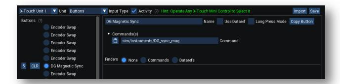
**Note:** If the encoder is operating a dual mode you will not be able to enter a command definition for the encoder's button since the button is used exclusively to swap between the inner and outer knob definitions for the dual encoder or to actuate a command in long press mode which gets defined on the encoder definition.
