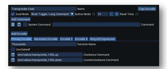
In this example we used the Add Encoder button to add Encoder 3 and Encoder 4 to the transponder dual encoder configuration. The primary encoder handles the 1000's digits, Secondary handles the 100's, the 3<sup>rd</sup> handles the 10's, and the 4<sup>th</sup> handles the ones's.
